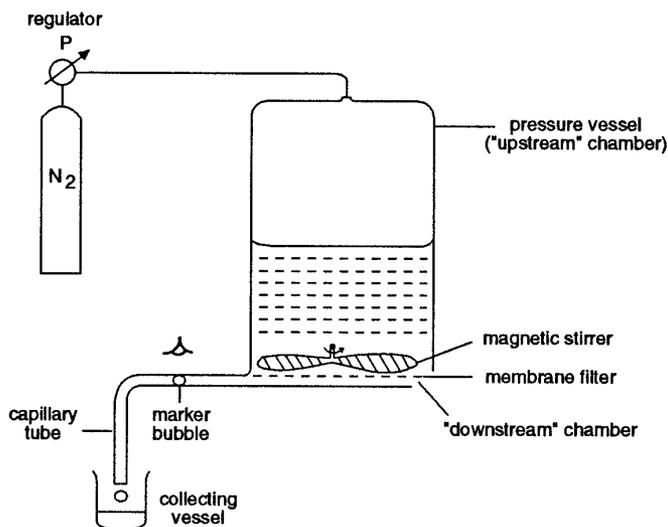
**FIG. 1.** Apparatus for measuring the osmotic pressure of PEG solutions.
