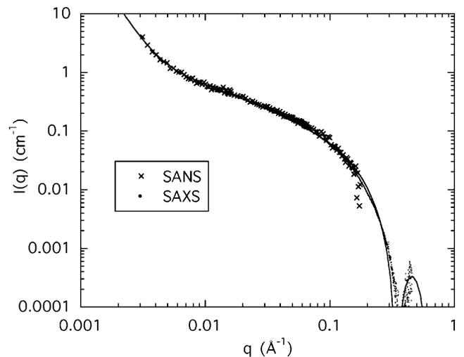
FIGURE 6 Normalized curves from SAXS at 15.8 keV and SANS for a 3% DNA solution in water containing 100 mM NaCl and 80 mM SrCl<sub>2</sub>. The SAXS data are converted to SANS contrast by multiplying the intensities by  $(\Delta\rho/r_0 K_p)^2 = 0.187$ , corresponding to Model 1. The continuous line is Eq. 4 where  $L = 200 \text{ \AA}$ ,  $r = 11.1 \text{ \AA}$ , and  $I(0) = 1.76 \text{ cm}^{-1}$ .
