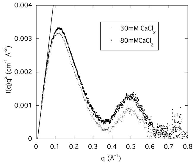
FIGURE 5 Kratky plot of the SAXS signals from a 3 wt % DNA solution containing 100 mM NaCl and either 30 mM CaCl<sub>2</sub> or 80 mM CaCl<sub>2</sub> at 14.900 keV. The straight line shown is the least-squares fit through the low  $q$ -data points, as described by Eq. 5.
