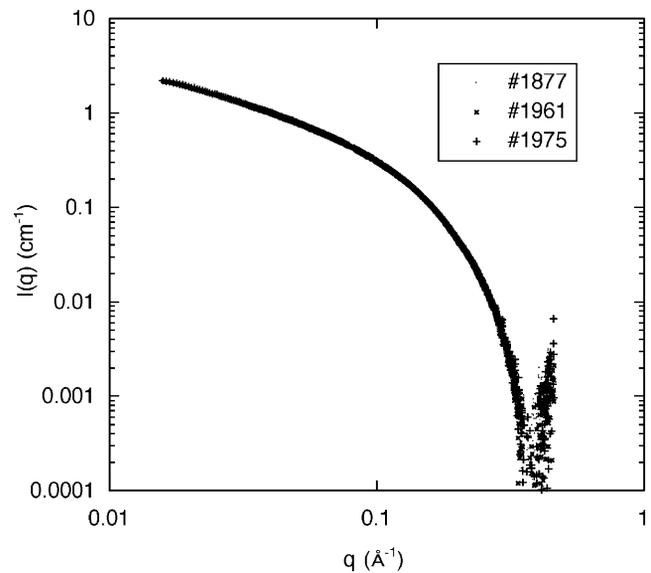
FIGURE 1 Scattering intensity at  $E = 15.8$  keV from a 3 wt % DNA solution containing 80 mM strontium chloride, in three successive exposures of 50 s at the same position in the sample. In this  $q$ -range, the responses are indistinguishable.
