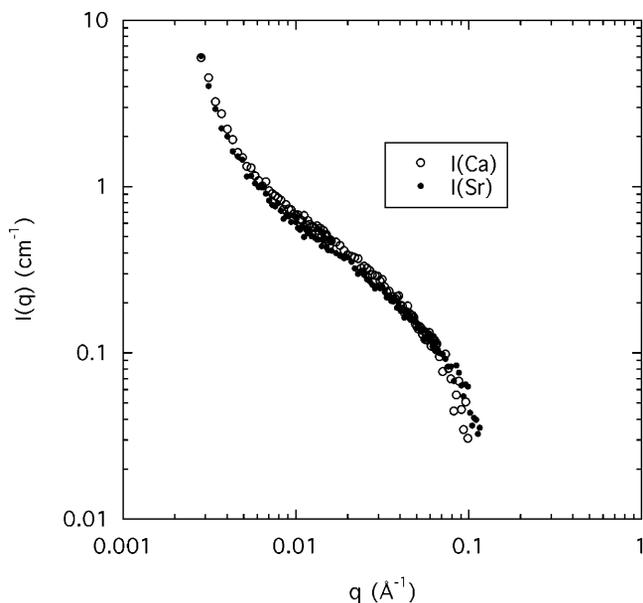
FIGURE 2 SANS response from a 3 wt % DNA solution containing 100 mM NaCl and 80 mM CaCl<sub>2</sub> (open symbols) or 80 mM SrCl<sub>2</sub> (solid symbols) in a 8% D<sub>2</sub>O/92% H<sub>2</sub>O mixture.
