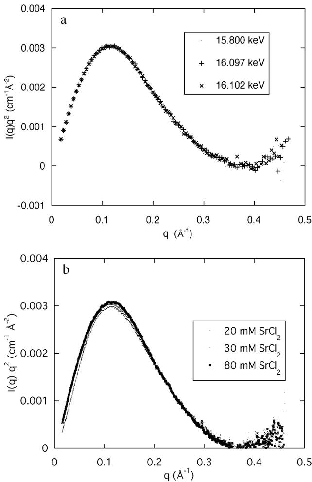
FIGURE 4 (a) Kratky plot of the SAXS signals from a 3 wt % DNA solution containing 100 mM NaCl and 80 mM SrCl<sub>2</sub> at 15.800 keV (■), 16.097 keV (+), and 16.102 keV (×). For clarity, only 10% of the data from each spectrum are plotted; (b) Kratky plot of the SAXS signals at 15.800 keV from three DNA solutions (3 wt %) containing 100 mM NaCl and 20 mM, 30 mM, and 80 mM SrCl<sub>2</sub> respectively.
