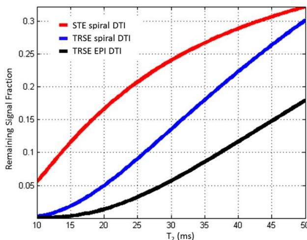
FIG. 5. Baseline signal fractions of water components with short  $T_2$  relaxation time constants for three MRI diffusion pulse sequences with  $b = 800$  s/mm<sup>2</sup> and minimum echo times: STE spiral DTI ( $TE = 22$  ms), TRSE spiral DTI ( $TE = 60$  ms), and the clinical TRSE EPI DTI ( $TE = 86$  ms) sequence, respectively. [Color figure can be viewed in the online issue, which is available at [wileyonlinelibrary.com](http://wileyonlinelibrary.com).]
