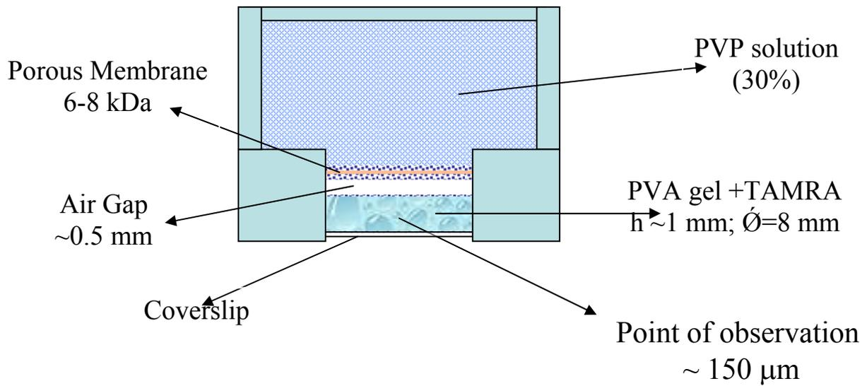
Figure 1: Schematic diagram of the optical chamber designed to study the effects of drying on nanoprobe diffusion in a gel.
