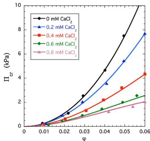
**Figure 4.** Osmotic pressure  $\Pi_{\text{cr}}$  versus DNA volume fraction  $\varphi$  for gels swollen in 100 mM NaCl solution containing different amounts of  $\text{CaCl}_2$ .
