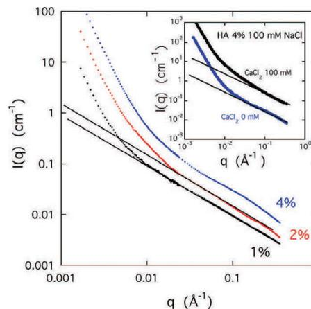
FIG. 5. SAXS curves for HA solutions at three concentrations in 100 mM NaCl. Inset: SAXS response of 4% HA solutions in 100 mM NaCl (lower curve) and in 100 mM NaCl+100 mM CaCl<sub>2</sub> (upper curve, shifted vertically by a factor of 10). In each part, the straight lines through the data points in the high  $q$  range have slope  $-1$ .
