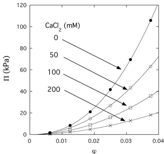
FIG. 2. Osmotic pressure dependence on the polymer volume fraction  $\varphi$  of HA solutions in 100 mM NaCl with different calcium chloride contents. Continuous curves are least-squares fits to Eq. (6). The  $\text{CaCl}_2$  concentration is indicated in the figure.
