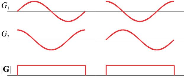
**Fig. 1.** *First two rows:* An RFG “pulse” involves two oscillating waveforms with a  $90^\circ$  phase shift applied simultaneously along two perpendicular directions. Our sequence involves two such pulses with a  $90^\circ$  phase shift. *Bottom row:* The magnitude profile of the RFG pulse sequence is identical to that of the traditional Stejskal-Tanner pulse sequence.
