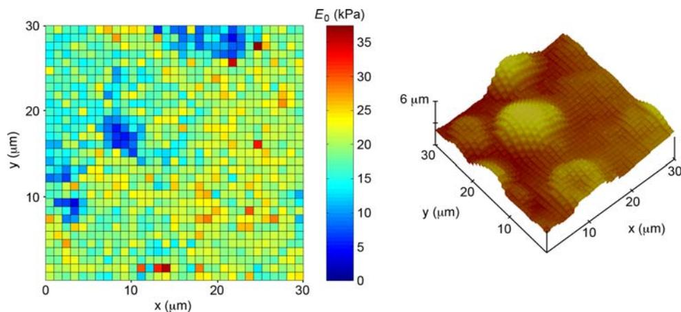
**Fig. 6** Young's modulus map and surface plot of a  $30 \times 30 \mu\text{m}$  region of mouse cartilage. Moduli were computed using the Fung model. Mean coefficient of determination of the 1,024 fits: 0.999
