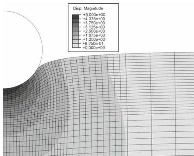
**Fig. 1** Finite element displacement magnitude map at the maximum displacement of  $5\ \mu\text{m}$ . The radius of the sphere is also  $5\ \mu\text{m}$ . The gradation of mesh size and the point at which the contact radius is measured are clearly seen
