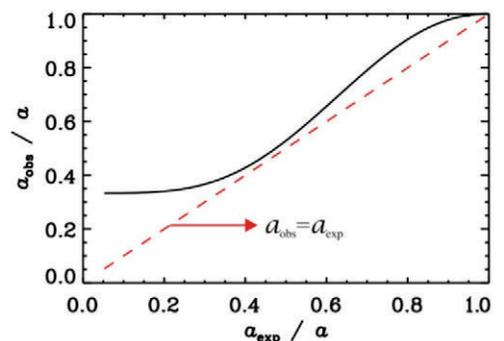
Figure 4. The pore radius observed under the assumption of circular cross sections against the radius of the circle that provides the correct value for the cross sectional area.
