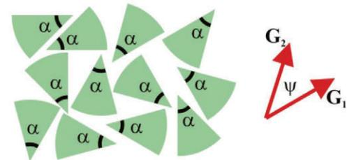
Figure 2. The specimen considered in this study includes a distribution of parallel tubes with randomly oriented asymmetric cross sections, where each compartment's cross section is a sector of a circle defined by the angle  $\alpha$ . The two gradients of the double-PFG sequence are applied on the same plane with the sectors.
