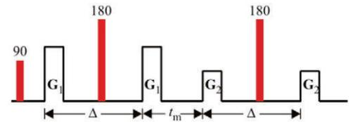
Figure 1. The double-PFG MR pulse sequence involves two pairs of gradient vectors where the time delay between the two pairs is called the mixing time,  $t_m$ .
