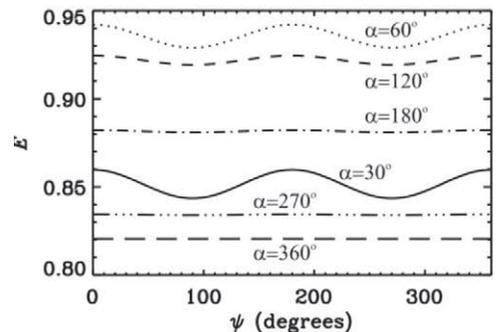
Figure 3. The double-PFG signal intensity plotted against the angle between the two gradients for varying values of  $\alpha$ .
