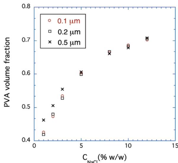
**Figure 3.** PVA volume fraction as a function of NaCl concentration in the equilibrium bath at  $25^\circ\text{C}$ .
