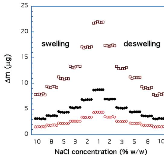
**Figure 2.** Equilibrium amount of absorbed water,  $\Delta m$ , as a function of NaCl concentration in the equilibrium bath at  $25^\circ\text{C}$  for the PVA samples shown in Figure 1.
