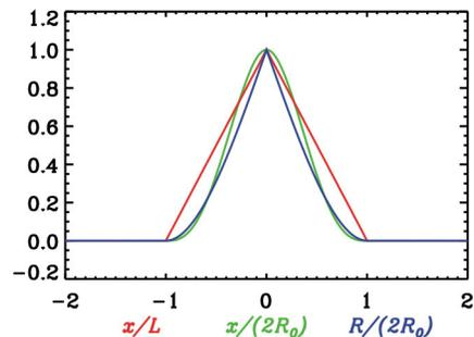
Fig. 3. The one-dimensional propagators for diffusion taking place between two parallel plates separated by  $L$  (red) and inside a spherical pore of radius  $R_0$  (green). The blue curve is produced by employing the three-dimensional isotropic transform to the signal for the spherical pore.
